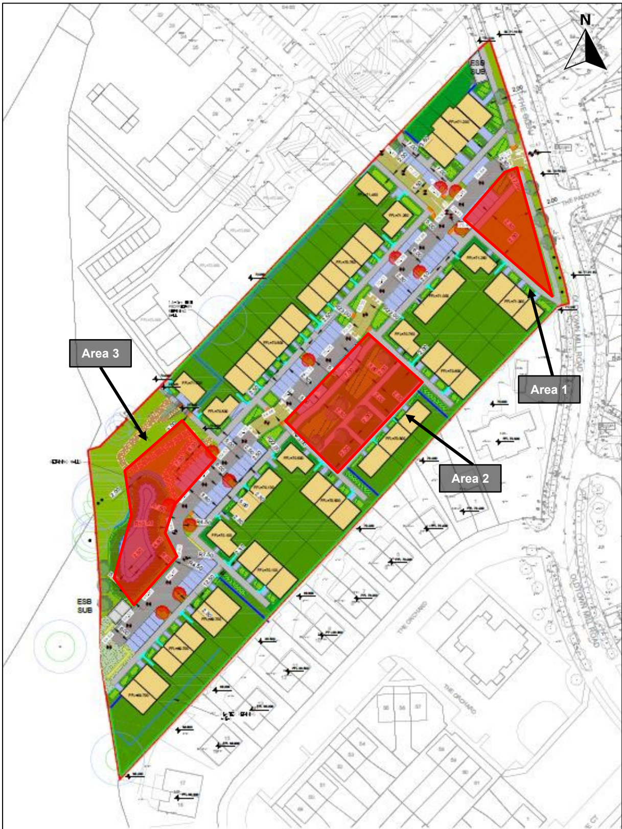
Figure 3.2: Possible Site Compound Locations
